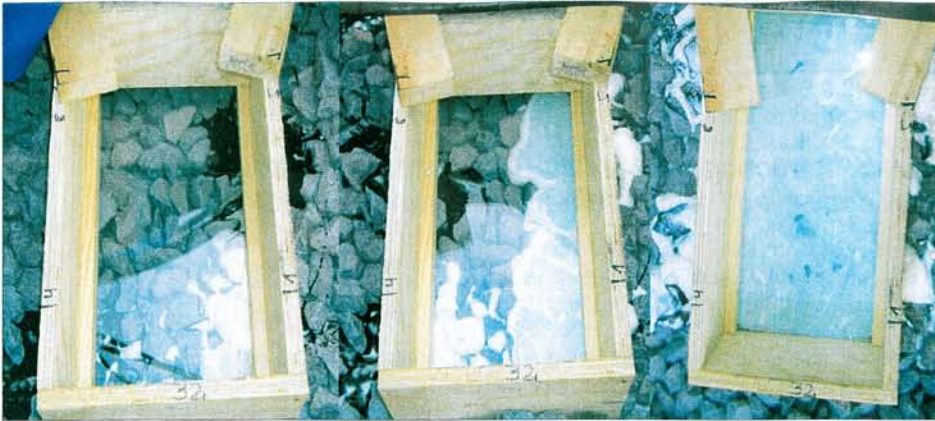
Fig. 2: The foaming result seen under a glass sleeper
