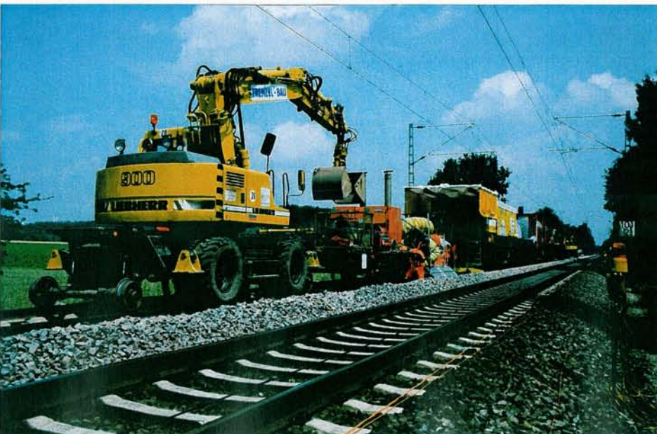
Fig. 4: Prototype of the foam-applying train
